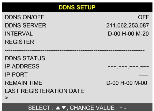
5) Go down to REGISTER and push ENTER button to renew IP and Port resistered on DDNS Sever(www.j2kip.com)
